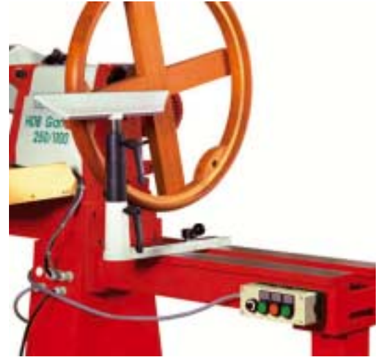
Headstock swivelled for outside-turnings 2nd bed can be retrofitted
