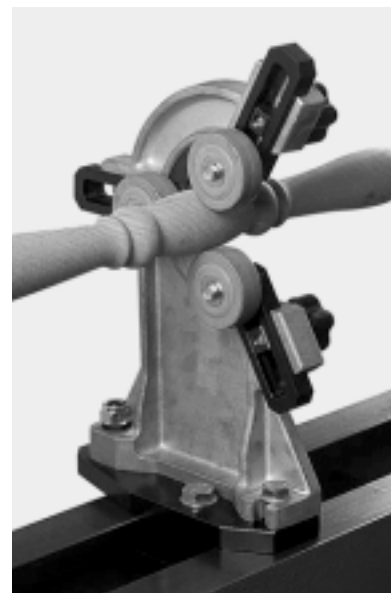
Lünette (nur für Handdreheln) Back rest (only for turning by hand)
